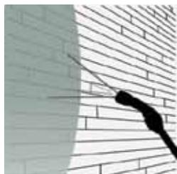
**STEP 2.** 1 bar of pressure should be sufficient. Spray evenly onto the surfaces.
