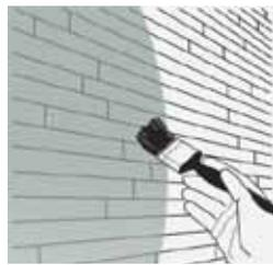
**STEP 2.** Brush evenly onto the stone surfaces making sure to work the sealer into the edges.
