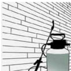
**STEP 1.** Ensure surface are as dry as possible. Fill a light pressure sprayer with the sealing solution.
