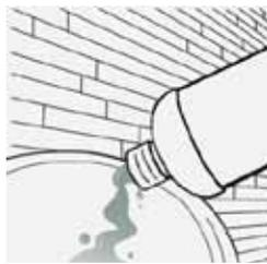
**STEP 1.** Ensure surface are as dry as possible. Fill a separate container with the sealing solution.
