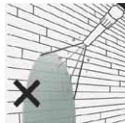
**STEP 5.** Keep dry for at least 3 days following application. Do not wash or make excessively wet.
